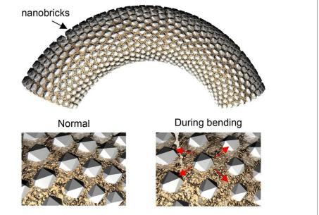
The nanometer size of the calcite bricks facilitates bending of the synthetic spicules. The radius of curvature upon bending is very large compared to the size of the individual particles. This prevents a fracture of the brittle mineral bricks.
